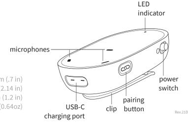
Height: 18mm (.7 in) Depth: 55mm (2.14 in) Width: 30mm (1.2 in) Weight: 18g (0.64oz)
