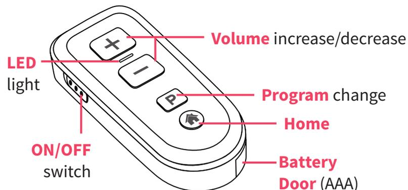
Turn ON your remote by sliding the **switch up**, and the LED light will **flash green** for 2 seconds. A **red flash** indicates low battery. To turn OFF, slide the switch down.
