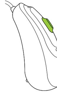
The device button controls the hearing aid volume. Both hearing aids are adjusted simultaneously. Turning off or charging will reset the device to the **default volume**
